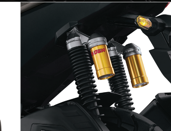
TWIN REAR SUSPENSION with SUBTANK
