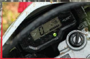
DIGITAL METER PANEL
